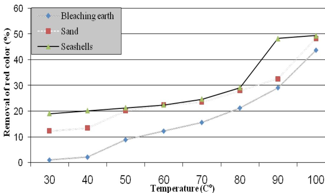
**Fig. 2.** Effect of Temperature (°C) on removal of red color (%) of crude soybean oil treated with seashells, sand and bleaching earth powders.
