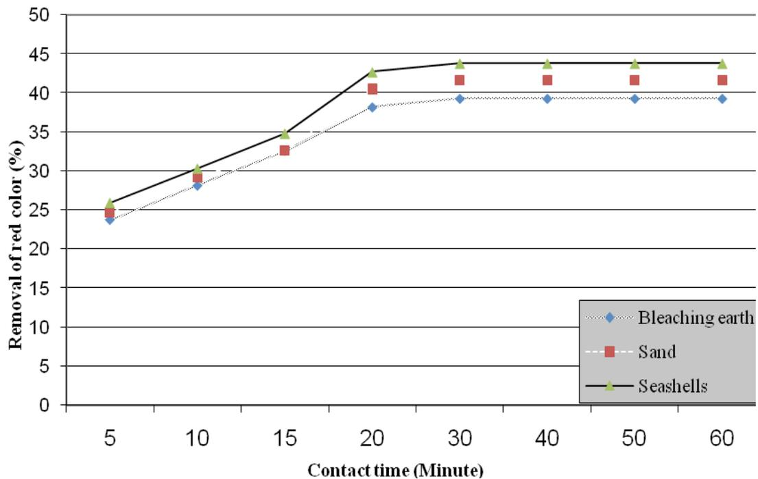
**Fig.1.** Effect of contact time on removal of red color (%)of crude soybean oil treated with seashells, sand and bleaching earth powders .
